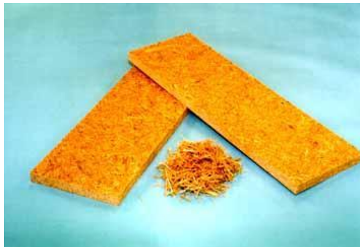
Bamboo Particle Board (Source: Shibusawa & Kin, 1996)
