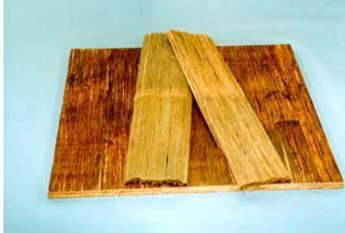
Bamboo Zephyr Board (Source: Sibusawa & Kin,1996)
